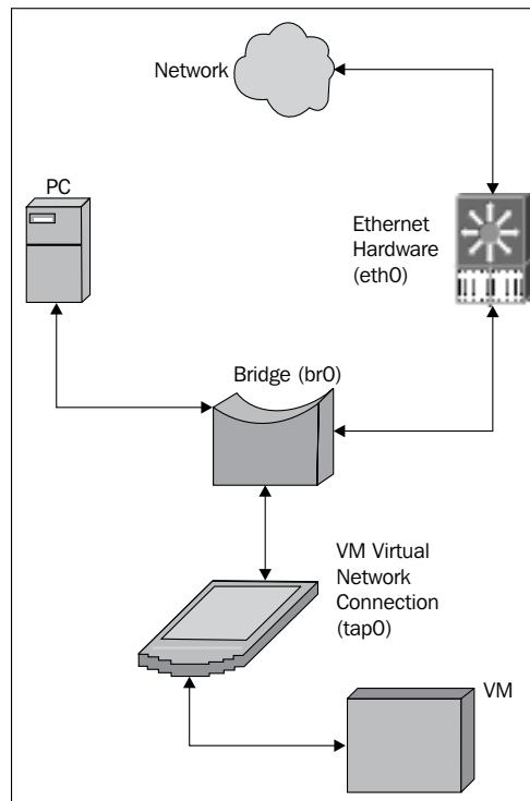
Note that the host machine now uses **br0** instead of **eth0** as its primary interface. The bridge interface uses **eth0** to connect to the actual network. The **VM (Virtual Machine)** will set up its own network interface (or you will set it up). These are generally set up as a tap or tunnel interface (hence the name **tap0**).
