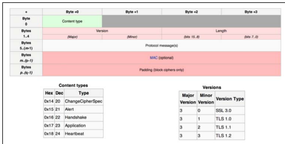
Figure 12-2. TLS record format, content types, and protocol versions
