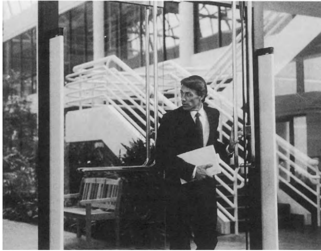
FIGURE 18-4 Sen Trac ID uses radio-frequency identification technology to provide hands-free access control and asset management to track people and products within a facility. Courtesy: Sensormatic.
