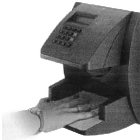
FIGURE 7-5 Verifying identity through hand geometry. Courtesy: HID Corporation.
