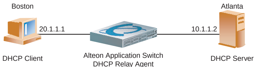
Figure 5-3 DHCP Relay Agent Configuration
