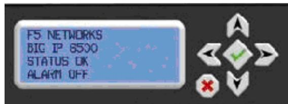
*Figure 2.1 An example of the LCD panel and control buttons*
