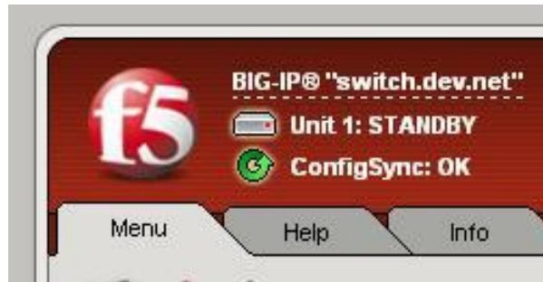
**Figure 13.3** Viewing redundancy state and synchronization status
