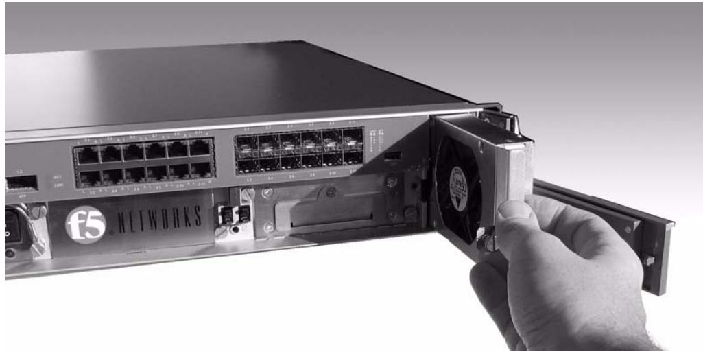
**Figure 5.1** The removable fan and filter tray
