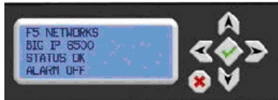
*Figure 3.1 An example of the LCD panel and control buttons*
