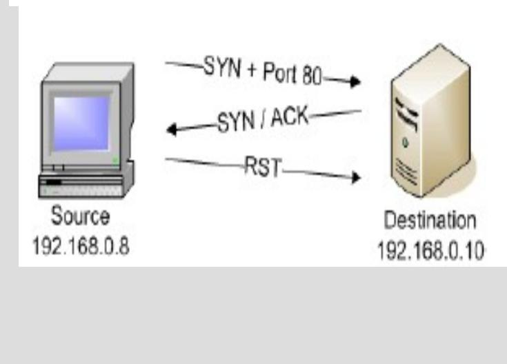
After the TCP SYN scan identifies port 80 as open, the version detection process begins. The process shown in this example is for this specific example. Other ports and application will operate differently.
